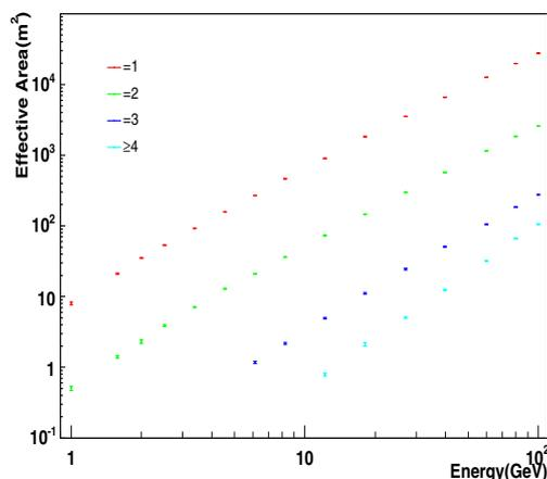
Figure 6. Effective area Vs. energy of 4 multiplicity channels =1,=2,=3,≥ 4
