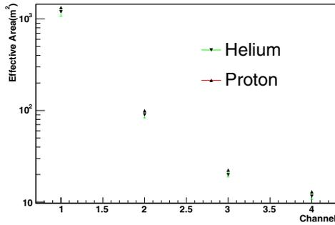
Figure 4. effective area for  $ch1(\geq 1), ch2(\geq 2), ch3(\geq 3), ch4(\geq 4)$  of the ARGO-YBJ experiment operated in scaler mode
