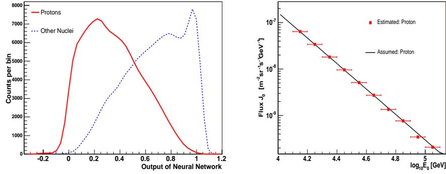
**Fig. 2.** Left: ANN output distribution of the proton-induced showers and other nuclei induced showers respectively. Right: Comparison between the assumed and estimated spectrum of protons. Only statistic error is taken into account here.
