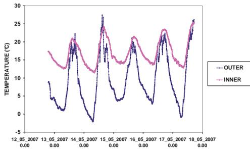
Figure 2: 5-day-long behaviors for the outer temperature and the inner temperature close to the RPC-carpet center, in May 2007.
