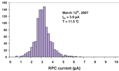
Figure 6: Single-chamber current distribution for 1400 RPCs of the ARGO-YBJ carpet.
