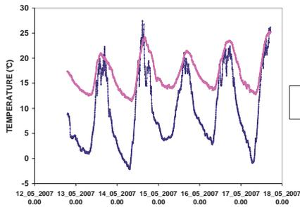
Figure 2: 5-day-long behaviors for the outer temperature and the inner temperature close to the RPC-carpet center, in May 2007.
