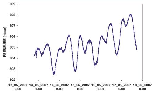
Figure 4: 5-day-long behavior for the barometric pressure at the ARGO-YBJ experimental site.
