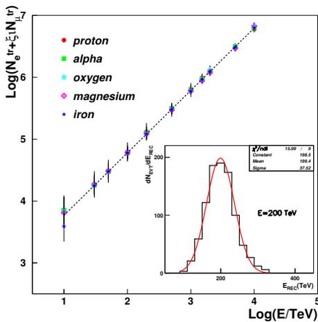
Fig. 1. Energy calibration; the error bars represent the size spread. Small frame: distribution of the reconstructed energies at 200 TeV.
