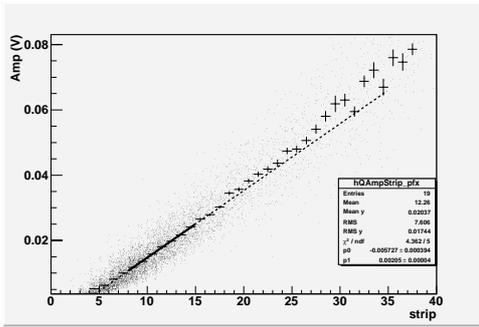
Figure 4: Single BP amplitude versus number of strips; the fit has been performed in the range 8-15 strips (heavy line).
