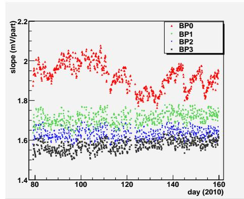
Figure 6: Gain behavior in 70 days of the 4 BP in a bicamera.
